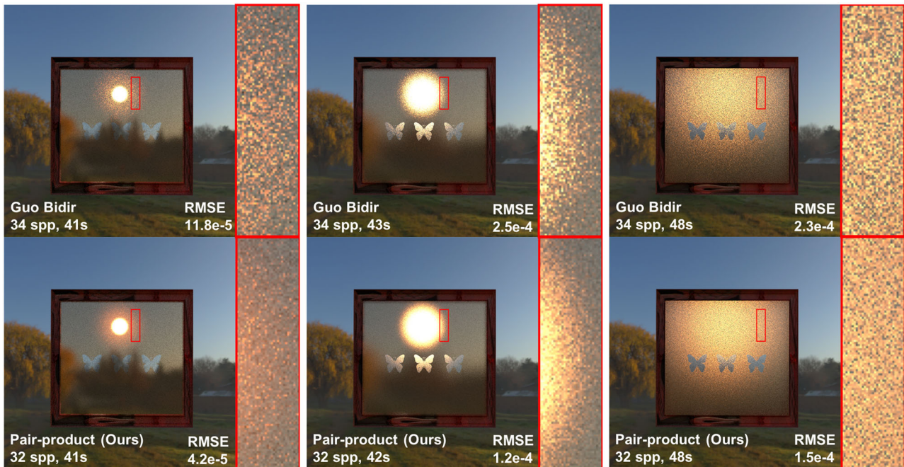
Figure 12: This scene contains a triple transmissive layer material (the framed area) with textured albedo and roughness. The scene is rendered using Guo et al.’s bidirectional (top row) and our pair-product sampling (bottom row). We rendered global illumination and the full path length through the layer stack. The red box shows the zoom area and is also used to calculate RMSE. The pair-product sampling obtains 1.5x to 2.9x reduction in RMSE, which corresponds to 2.3x to 8.4x reduction in render time.
