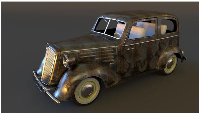
Figure 11: A double textured layer car scene rendered using our pair-product sampling strategy. The top layer uses procedural noise to texture the roughness, and the bottom layer uses image maps to texture albedo and roughness. We rendered global illumination and the full path length through the layer stack with 1024 spp. The running time is 46 min.
