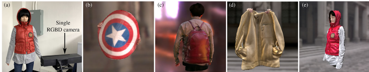
Figure 1: (a) We provide the first-ever method to simultaneously estimate the SVBRDF, shape and motion of dynamic objects using a single RGBD camera. (b)–(e) We obtain both diffuse and specular appearance with our novel joint optimization scheme, based on our hierarchical data structure, which allows us to render captured scenes under novel view and light conditions. Refer to the supplemental video for more results.
