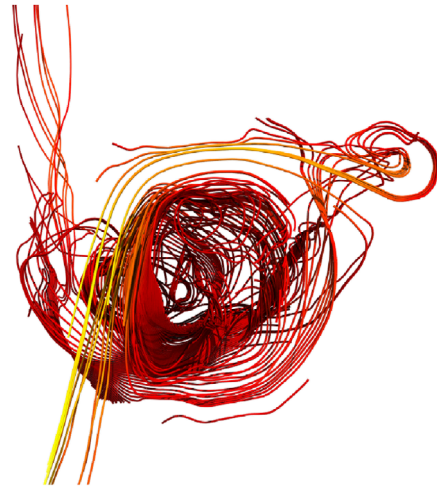
Figure 5: Streamlines of the measured flow before our method was applied. All visualization parameters (number of lines, seeding position and cutting plane) are equal to those in Figure 6. Note the presence of a vortex in the top-right corner and the helical flow present in the top-left corner and from the centre towards the top-right corner.
