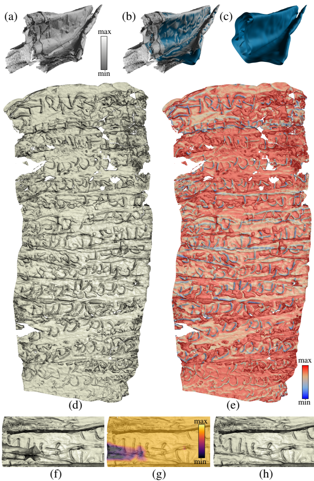
Figure 8: Silver scroll: (a) volume rendering of \mu CT image; (b) same as (a) with M_{\text{curv}} ; (c) M_{\text{curv}} ; (d) thin iso-surface rendering; (e) thin iso-surface rendering with distance to M_{\text{curv}} color-coded (blue=behind, red=in front of M_{\text{curv}} ); (f) zoom-in with occluding structure; (g) modified ray length color-coded; (h) occluding structure partially removed.
