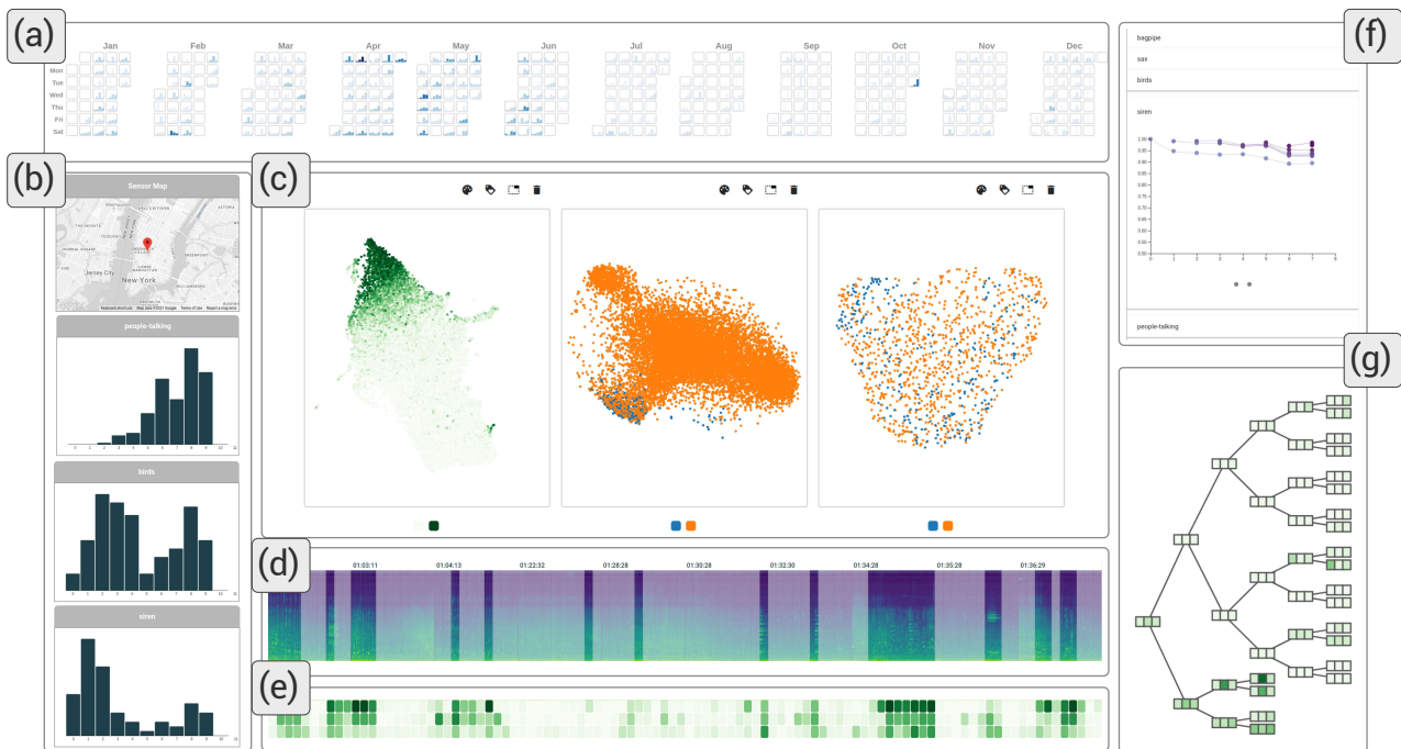
Figure 3: The Urban Rhapsody system visual interface: (a) Calendar View; (b) Sensor Map and Distribution View; (c) Day View (projections); (d) Focused View (spectrograms); (e) Frame Classification View; (f) Model Summary; (g) Mixture Explorer.
