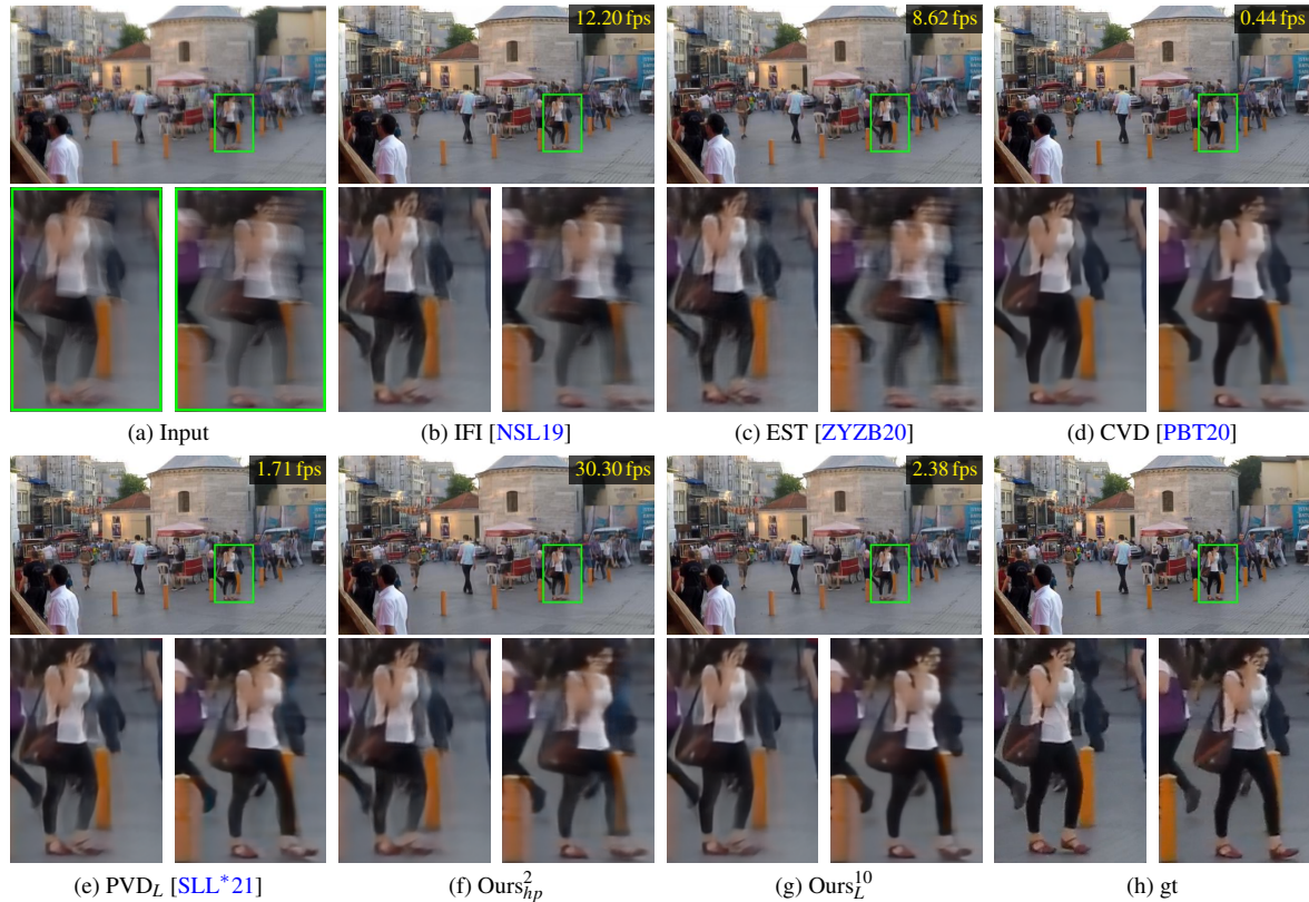
Figure 8: Comparison on the GoPro dataset [NKL17]. Cropped images visualize regions in the green box of two consecutive frames.
