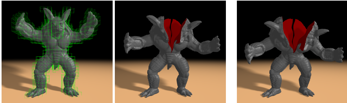
Figure 4.7: Left: The coarse hexahedral simulation grid and the high-resolution surface that is constructed from the embedded fine grid. Middle: Simulation using composite elements obtained from coarsening the hexahedral finite element model by three levels (10,563 DOFs). Each simulation time step takes 176.37 ms. Right: Simulation of cuts in the Armadillo model using hexahedral finite elements (569,748 DOFs). Each simulation time step takes 2829.87 ms.
