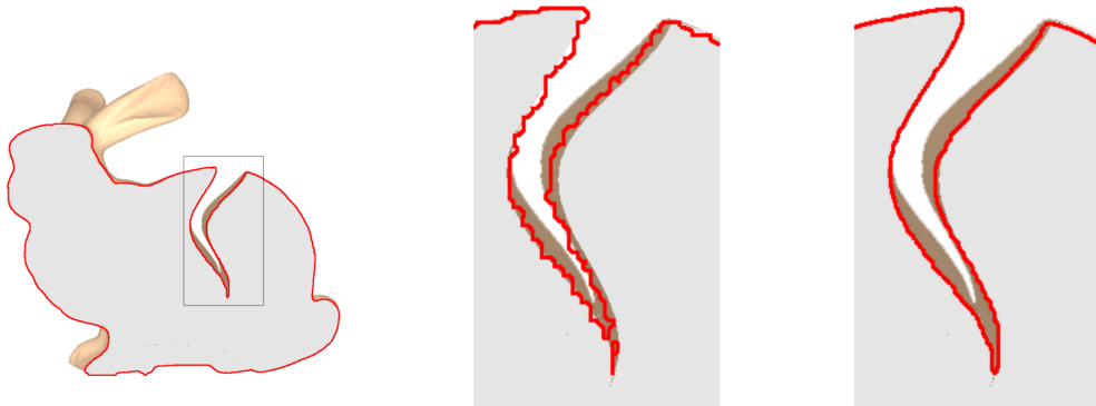
Figure 5.5: Comparison between the zero isocontours of the distance fields obtained by the simple interpolation approach (middle) and our topology-aware interpolation approach (right).
