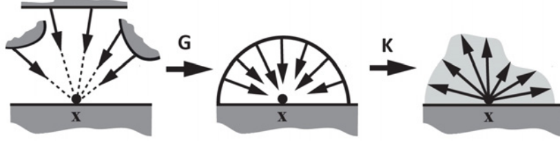
Figure 2.3: The actions of \mathbf{G} and \mathbf{K} at a single point \mathbf{x} . The operator \mathbf{G} converts exitant surface radiance ( left ) directed toward \mathbf{x} into incoming radiance ( middle ), where it is again mapped into exitant surface radiance by the reflection operator \mathbf{K} ( right ).
