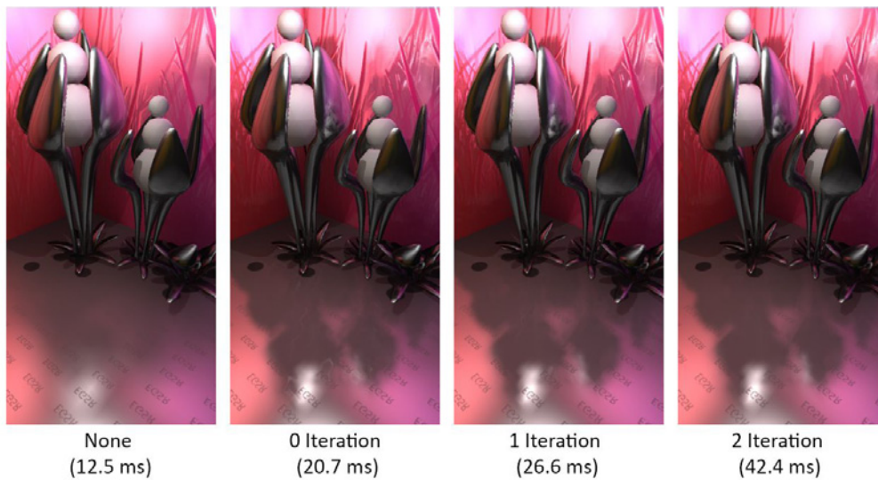
Figure 3.10: None, as well as different numbers of recursion, ( left to right ) for an glossy ground plane. It can be seen, that after no or one iterations, the lookups for the purpose of glossy reflections in Radiance Caching are sufficiently accurate. Note, that the overlap between splats smooths out errors. Consequently, the error appears as blur, instead of noise or banding. A successful lookup, such as ours, will result in sharp reflections.
