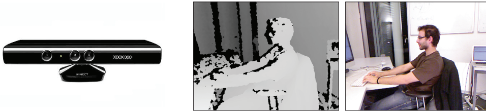
Figure 4.4.: The Kinect simultaneously captures a 640 \times 400 color image and corresponding depth map at 30 Hertz, computed via triangulation of an infrared projector and camera.
