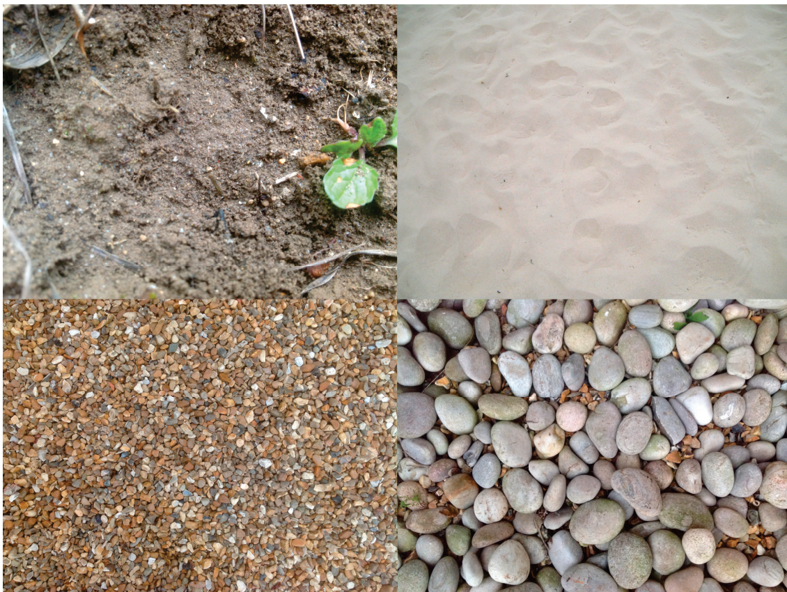
Figure 1.3. Four examples of terrain grains sizes as classified by Wentworth [26]. Top left: silt; Top right: sand [27]; Bottom left: gravel soil - granule; Bottom right: gravel soil - pebbles;
