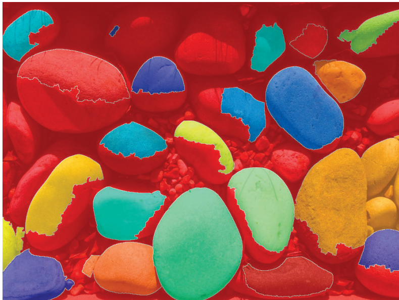
Figure 3.7. Output from the watershed algorithm with automatic labelling applied to figure 3.4. The red area is identified as background by the algorithm, coloured areas are identified as foreground.
