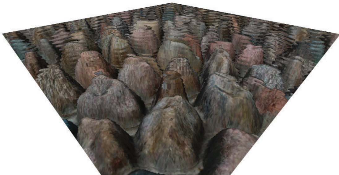
Figure 2.7. Example of parallax mapping failing, notice that the edges of the mesh are straight instead of following the curves of the stones and the ripples caused by the low camera angle with respect to the terrain
