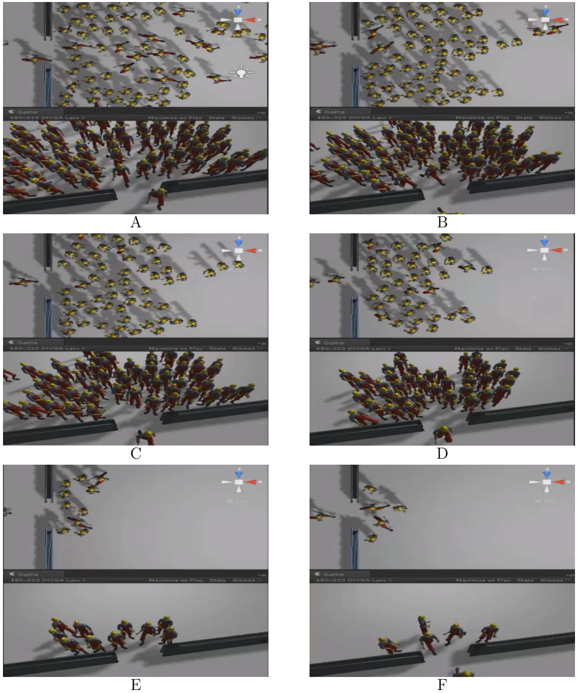
Figure 6.12: Rendered scenes of the simulation for the closed room with an exit experiment with the ITVQQL schema and 90 agents. The images are divided in two views of the same scene. The temporal sequence of stills is sorted alphabetically.
