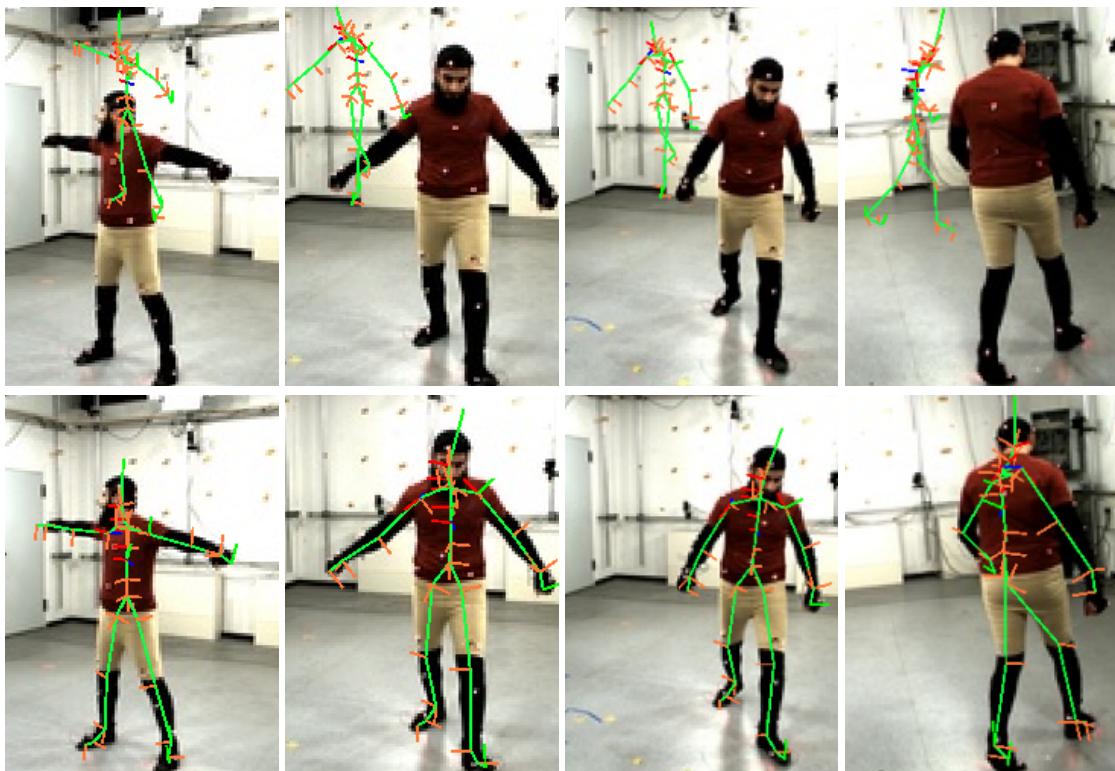
Figure 6.12: Comparison with [Stoll et al. (2011)] on a moving and static cameras sequence ( Walk 6 ). Four sample frames of the tracking result from one moving camera view. Top : [Stoll et al. (2011)]; average error 25.9 (pixel). Bottom : Our algorithm; average error 1.8 (pixel).
