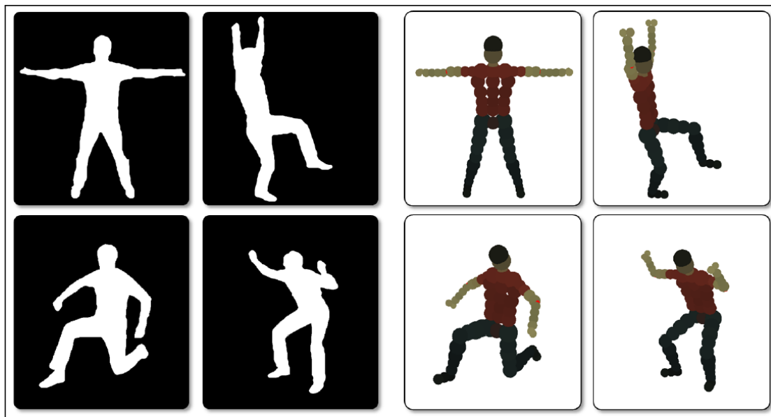
Figure 3.4: Estimating an actor specific model from example pose images. Left: Single segmented input image of the multi-view sets for each pose. Right: Resulting actor-specific body model after optimization and color estimation. [Stoll et al. (2011)]
