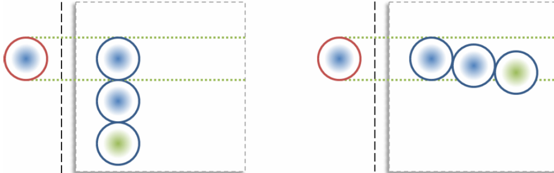
Figure 3.6: Self-occlusion approximation. Inside boxes: Top view of 3D model SoG. Left of dotted line: Image plane with 2D Gaussian. Left column (no occlusion): As long as no occlusions happen, (Eq. 3.2) calculates a correct overlap of a single element. In this example, the color (blue) and the shape are identical, yielding the similarity E_{ii} . Right column (occlusion approximation): If several 3D model Gaussians project to the same screen space coordinate, their contribution is cumulative, yielding a similarity larger than E_{ii} , even though two of the model Gaussians should be occluded. Using (Eq. 3.6) correctly limits the contribution of a single 2D image Gaussian, yielding the same similarity E_{ii} for both cases. [Stoll et al. (2011)]
