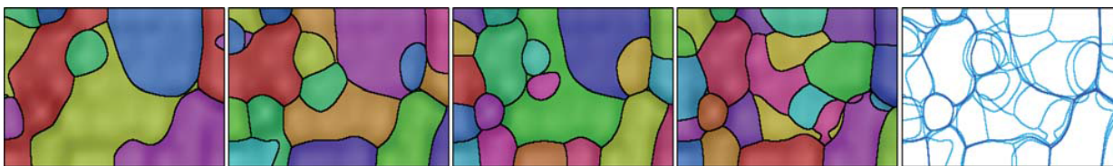
Figure 5.13 Four cluster correspondence visualizations facilitating the k-means algorithm. The clustering results of different parameterizations ( k = 5 , k = 10 , k = 20 , and k = 30 ) can be compared. On the right, the cluster borders of all four clusterings are shown via superposition, revealing recurring cluster border patterns. The user is able to estimate a) the number of clusters of the data set and b) the appropriate parameterization for the k-means algorithm.
