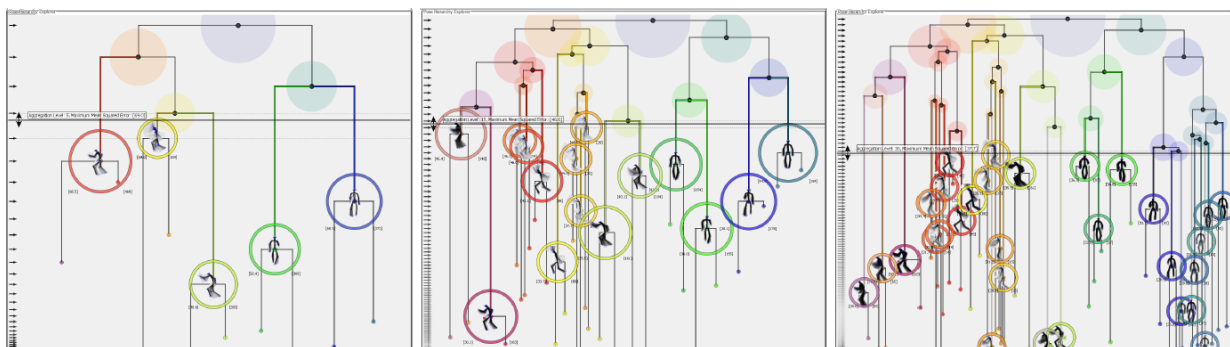
Figure 5.24 The result of a hierarchical clustering is shown in a tree-based visualization. Domain experts can change the level of abstraction by dragging the aggregation level slider. Here, poses of skiing movement are drilled-down to the aggregation levels of 5, 15, and 30.
