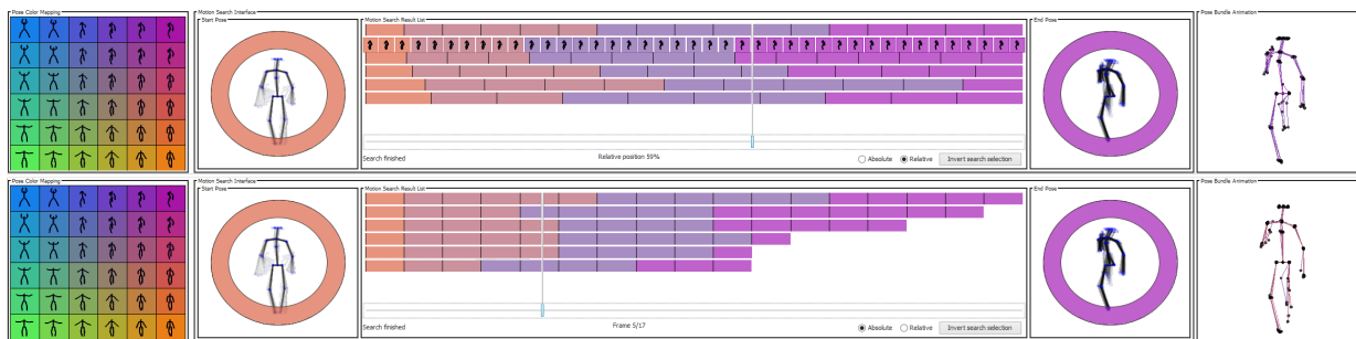
Figure 5.29 The search interface of the MotionExplorer system presented in Section 7.2. The user is able to define a start and an end pose. As a result, the retrieval algorithm of the MotionExplorer system is executed revealing a set of human motion sequences. The visualization and interaction design of MotionExplorer allows exploring the result set in detail. Users can switch between an absolute time axis meaning that the temporal domain of every retrieved sequence has an equal length or relative time axis where all sequences are stretched to the full length of the result visualization.
