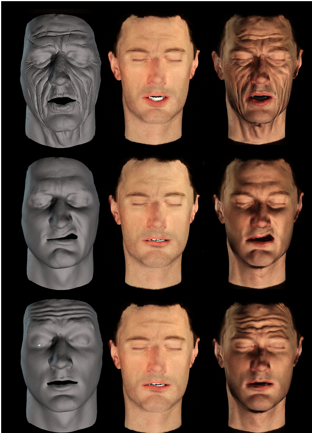
Figure 5.10: Three captured results of extreme poses, generated with our system. For every frame, the desired appearance is on the left, the robot configuration under uniform white illumination is in the middle, while the augmented result is on the right.
