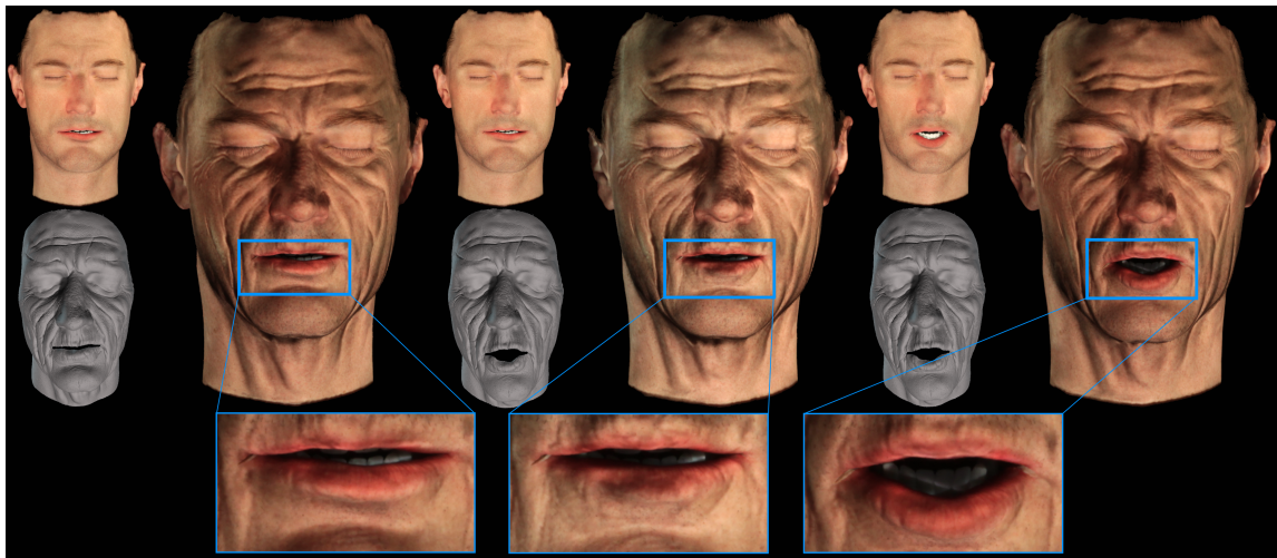
Figure 5.12: The neutral pose (left) of a sequence, compared to an extreme pose while the animatronic head is kept static (middle), and while it is actuated according to the proposed method (right). The head configuration under uniform illumination, and the target appearances are shown to the left of each result.
