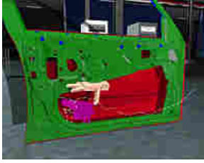
Figure 5.14: During assembly, the path of any part can be recorded, edited, and stored in the PDM system.
