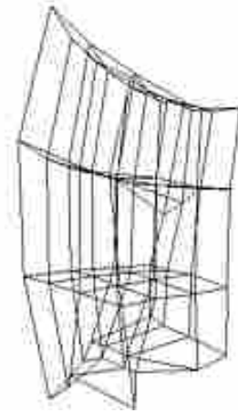
Figure 4.15: Another real-world field of one of our demo sites. The volume measured is about 1 \times 1 \times 2 \text{ m}^3 , the long-range transmitter was about 1 m above the ground.
