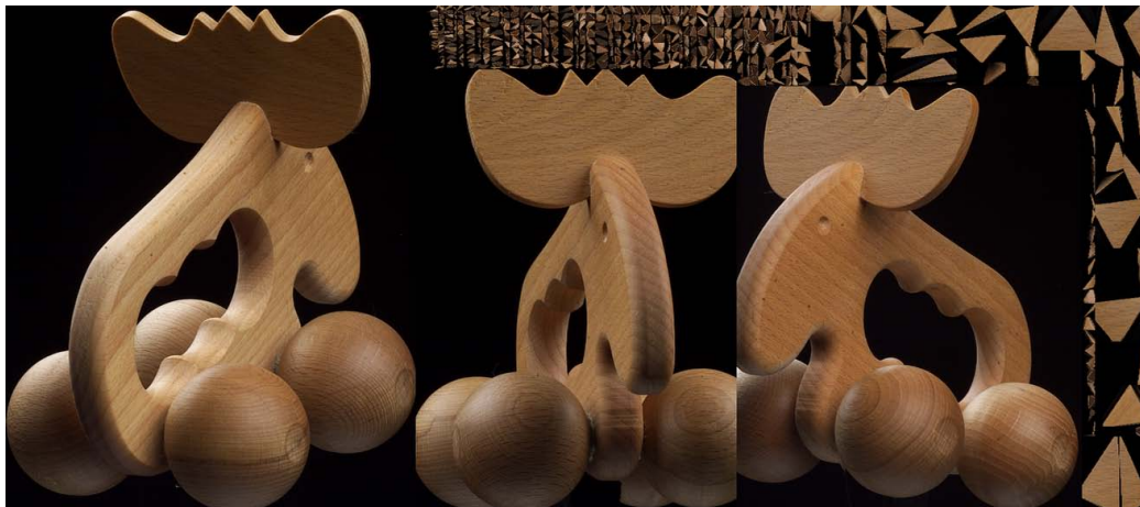
Figure 5.7: All image information of three images packed into a single texture. The texture consists of the relevant rectangular regions of the original images and of the blended textures for single triangles. (Although the final texture consists of 15 images, only three pictures were considered in this case to better visualize the layout of original image parts and blended triangles.)
