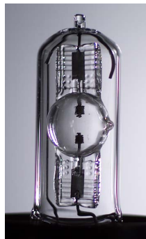
Figure 4.2: A HMI bulb mounted in a lamp. An electric arc is produced between the two electrodes in the inner glass ball. The effective light source diameter is smaller than 1 cm.
