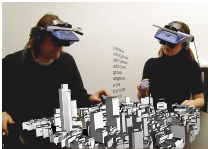
Figure 2.7: A typical augmented reality application for architectural planning. Image courtesy of the VR Center for the Built Environment [ VR Centre for the Built Environment 2004 ]
