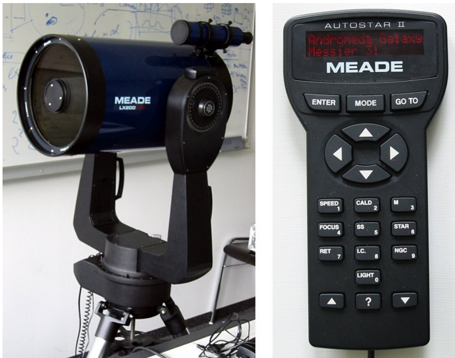
Figure 8.3: Left: The Meade LX200 GPS 10'' Astronomical Telescope used in the application. Right: The hand controller provided with the telescope
