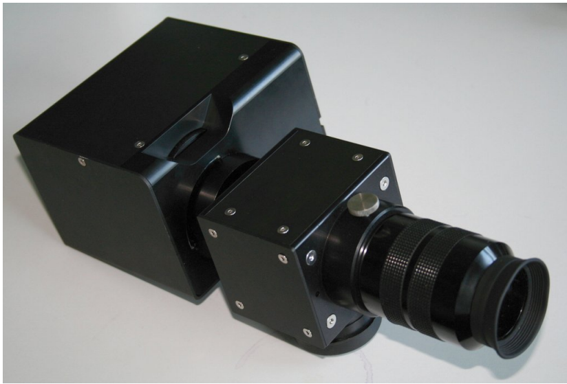
Figure 8.6: A photograph of the projection system together with the 32 mm eyepiece. It is directly mounted on the telescope's optical axis through the flange on the bottom side. The eyepieces in use are placed in the provided holder on the right side. The DLP engine and LED head are situated in the box on the left. The box in the middle contains the 45° mounted beam splitter
