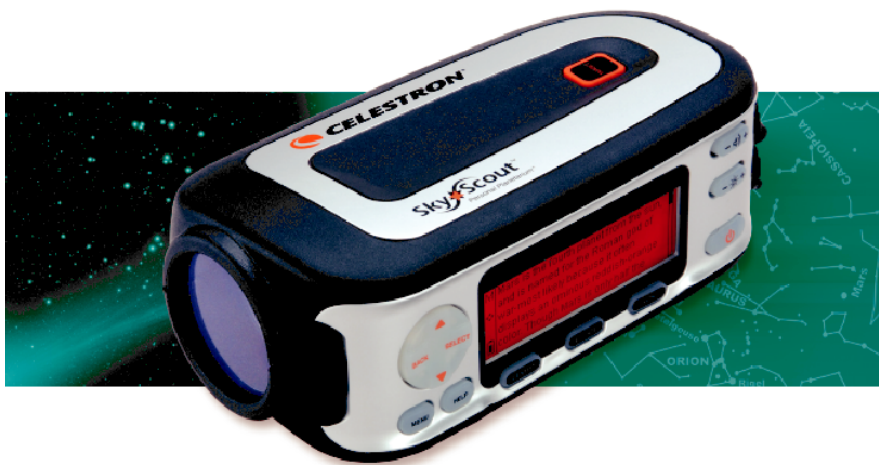
Figure 3.3: Celestron Sky Scout Personal Planetarium. The user selects a desired object, points the device to the sky and she / he is guided into the direction of the object by arrows inside the viewfinder. Additional information and audio guides for many astronomical objects are provided as well. Image courtesy of Celestron [Celestron, LLC. 2006]
