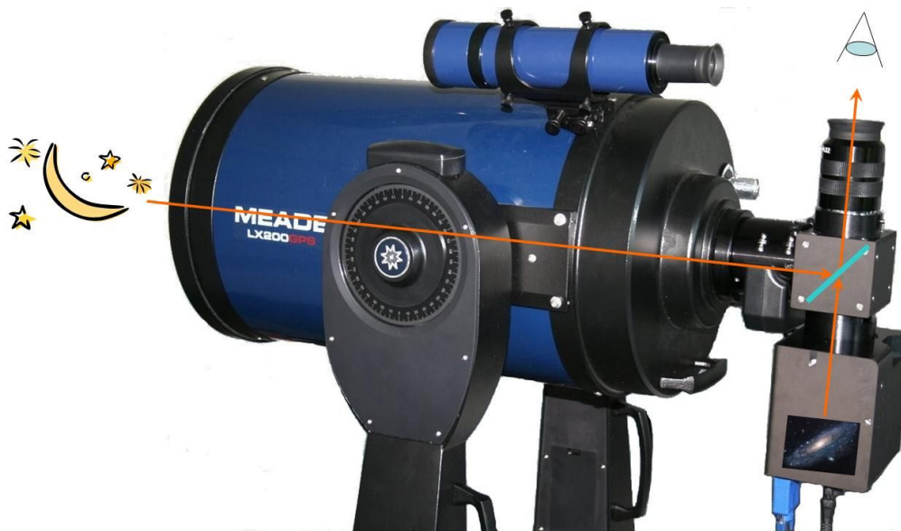
Figure 8.7: The projection unit together with an eyepiece mounted on the telescope. The figure also highlights the path light from the currently observed astronomical object and the projector travels. The beam splitter combines these images and the observer magnifies the final image using an eyepiece
