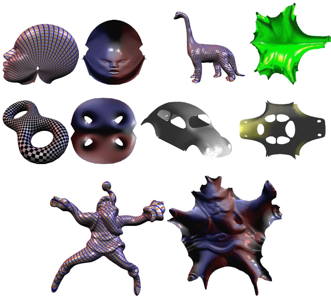
Figure 6.10: More maps computed with our method: The head model (16K \Delta ) self-intersects in 3D, the flat mesh shows no foldovers. Dinosaur (48K \Delta ). Double torus (2K \Delta ). Holes like the windows of the beetle model (2K \Delta ) do not require any special treatment. Santa (114K \Delta ).
