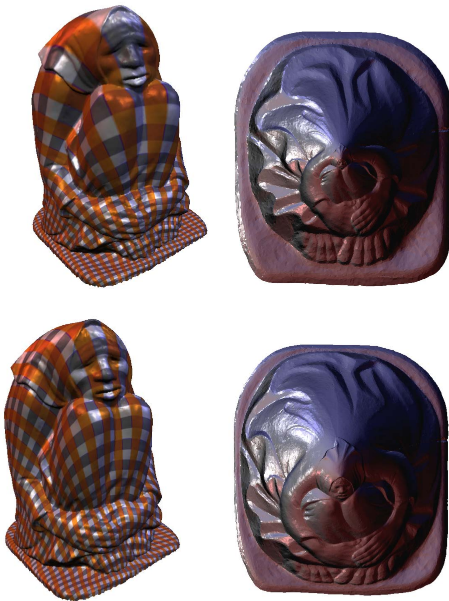
Figure 5.12: Maps of a sculpture (89KΔ). Left: Mean value coordinates. Right: Quasi-harmonic map. The mesh was obtained from a range scan of the wooden sculpture Freezing Old Woman (Frierende Alte, 1937) by the German expressionist sculptor Ernst Barlach (1870-1938).
