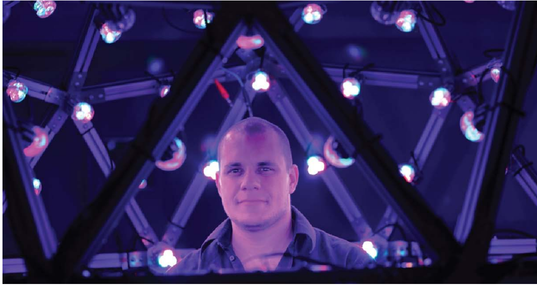
Figure 3.4: Helios is a versatile multi-purpose light stage, which can produce arbitrary spatio-temporal illumination.
