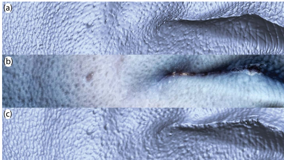
Figure 5.10: Qualitative comparison - Top: rendering of the physical mask; Center: image of the physical mask; Bottom: rendering of the recovered model.
