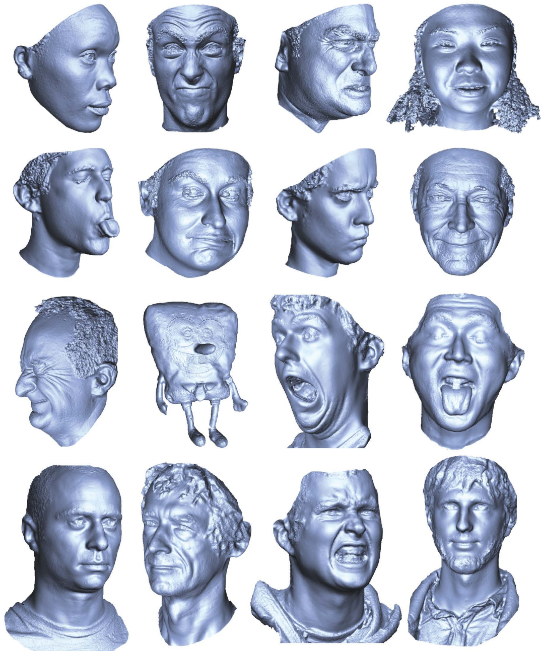
Figure 5.13: Recovered models and synthesized views, for viewpoints different from the original camera images, across subjects of varying appearance. Our focus has been on skin, and it may be that the hair and specular components — like the eyes, teeth and tongue — benefit from custom algorithms. But 3D reconstruction is reasonable across all these parts.
