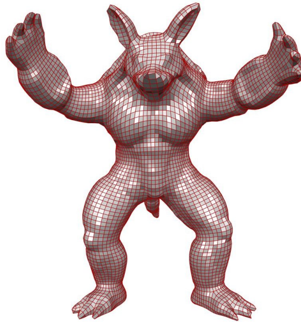
Figure 5.4.: A quadrangulation of the ARMADILLO model, used in our benchmarking. Its organic structure leads to more complicated optimization problems compared to designed mechanical objects.
