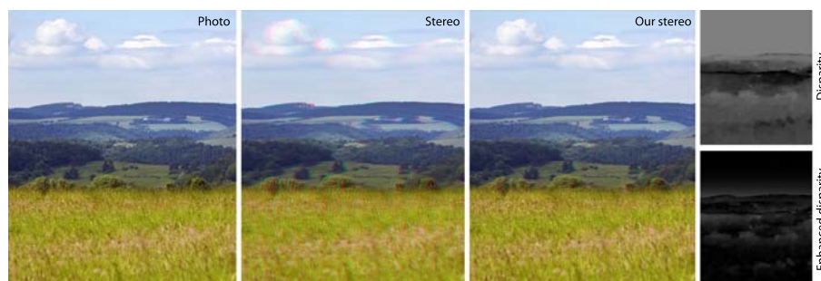
Figure 7.15: Converting a photo (Left) into a 3D image (Middle, anaglyph), just by using the blue channel as depth. Our enhancement (Right, anaglyph) can be used to put stereo cues only where depth contrast exists, minimizing the global error due to the naïve 3D reconstruction, but with locally plausible cues. The insets on the right depict the corresponding disparity maps.
