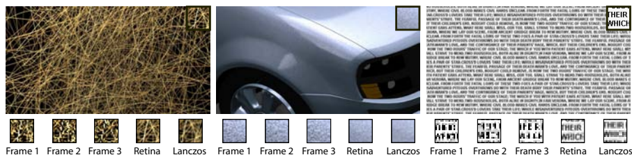
Figure 5.1: Depicting fine details such as hair (left), sparkling car paint (middle) or small text (right) on a typical display is challenging and often fails if the display resolution is insufficient. In this work, we show that smooth and continuous subpixel image motion can be used to increase the perceived resolution. By sequentially displaying varying intermediate images at the display resolution (as depicted in the bottom insets), subpixel details can be resolved at the retina in the region of interest due to fixational eye tracking of this region.
