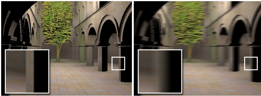
Figure 2.7: Simulation of hold-type blur. An animation sequence with the sample frame as shown on the left is displayed simultaneously with 60 and 120 Hz refresh rates on a Samsung 2233RZ 120 Hz display. The effective velocity of horizontal motion as seen on the screen is the same in both cases. The user’s task is to adjust the blur in the sequence refreshed with 120 Hz until the level of blur matches the 60 Hz sequence. The average outcome of such an experiment is shown on the right. In other words, the sequence of blurred frames (right) at 120 Hz are visually equivalent to the sequence of sharp frames (left) displayed at 60 Hz.
