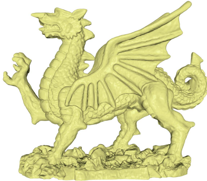
Figure 5.1: Welsh Dragon. We compress the 2.2 M triangles of the Welsh Dragon from 96 bpt to 3.72 bpt. It takes 1.6 ms for our data-parallel algorithm to decompress the mesh.
