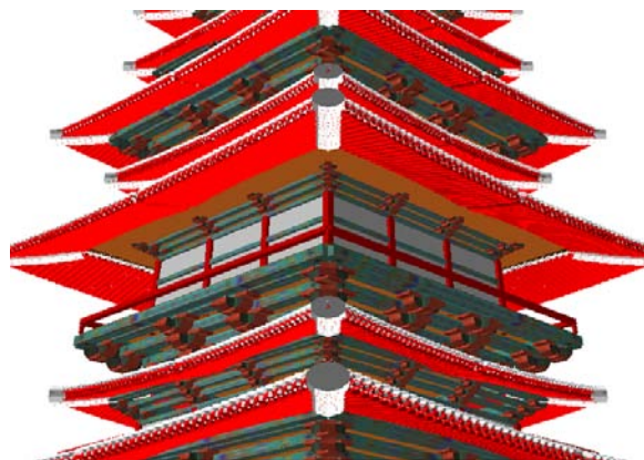
Figure 14: Colorful beams and brackets characteristic of Korean temple buildings. This example also shows a storey supported by bracketed beams.
