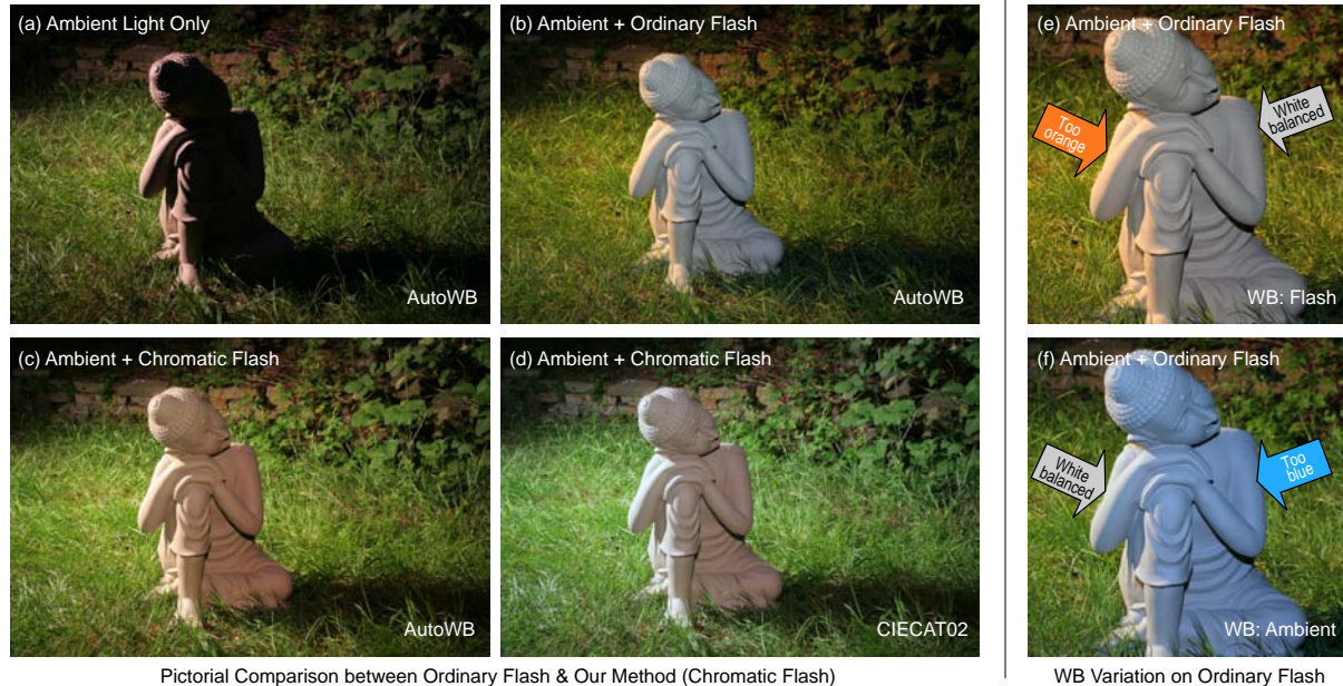
Figure 6: Image (a) is a photograph of a statue under the gas street lamp using ambient illumination only, lacking detail on the statue. Image (b) is captured with a flash unit, showing the mismatch of the ambient and auxiliary flash light – the statue stands out bluish from the warm environment. Images (c) and (d) is captured with the proposed chromatic flash (using different white-balancing algorithms for reference). Our chromatic flash (c and d) produces a consistent appearance and no visible mismatch in illumination. For completeness, images (e) and (f) show alternative white-balancing for the ordinary flash image: ambient for (e), and flash for (f). This results in a yellowish tint on the left of the statue for image (e) and overly bluish for image (f).
