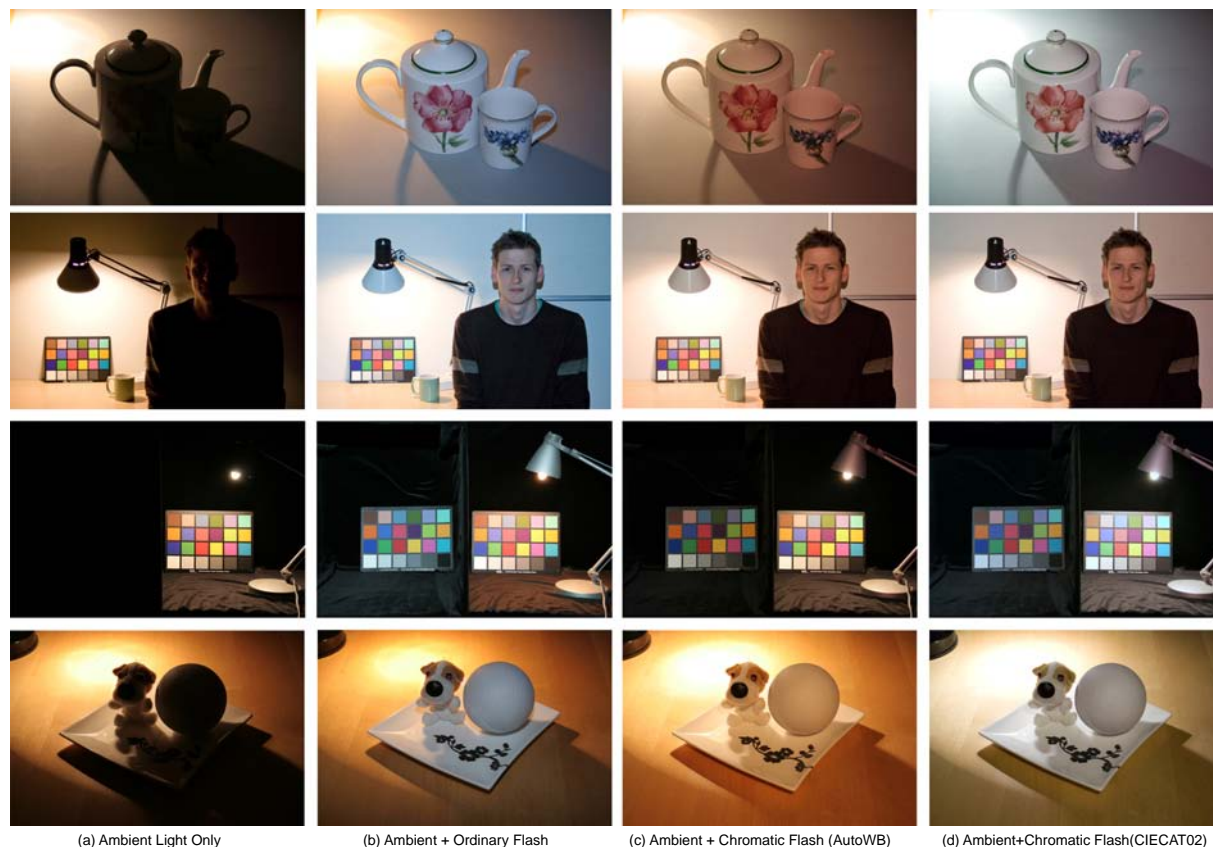
Figure 7: Results of our chromatic flash. Column (a) presents the captured image with ambient illumination only. Column (b) provides the results when using an ordinary flash unit with white balancing set to mixed illumination (ambient and flash). Flash illuminated areas appear relatively bluish. Column (c) is the result of our proposed method with camera auto white balancing, which preserves the atmosphere of original scene illumination. Column (d) is also the result of our proposed method but with manual white balancing (CIECAT02).
