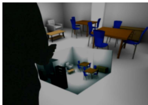
Figure 1: User interacting with the WIM. The non-dominant hand is used to establish the frame of reference by rotating the WIM, whereas selection and manipulation tasks are performed with the dominant hand.
