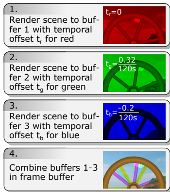
Figure 5: Simple rendering algorithm for 120Hz output without motion blur, using four passes. First, each color channel is rendered using the respective time offset for the animation. Finally, the channels are combined and written to the frame buffer.
