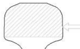
Figure 4: Inspected area in the rail head is hatched in the cross-section.
