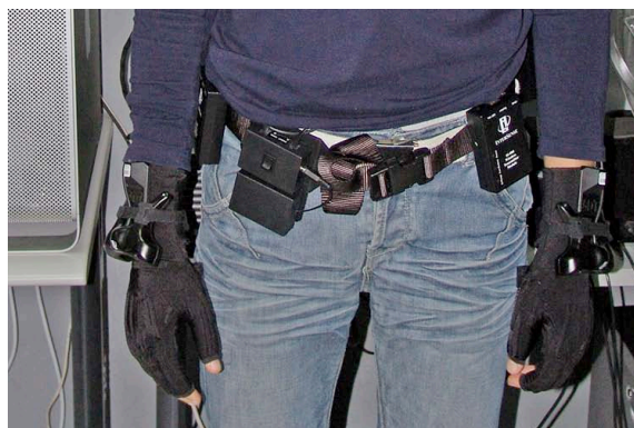
Figure 2. A user wearing left and right handed wireless instrumented gloves (Data Glove 14 ultra from 5DT) plus the IS-900/VET Inertial 6DOF Tracking system from Intersense used for wrists/head wireless motion tracking.
