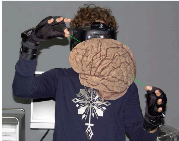
Figure 4 - User performing object rotation by means of two virtual handles corresponding to the extremities of the green vector. Due to the optical see-through design of the HMD this image is simulated as the scene was observed from a third person point of view. The brain model is the result of actual medical imaging processed to generate a 3D geometry and further optimized (about 625,000 triangles). The color texture shown is fictional.
