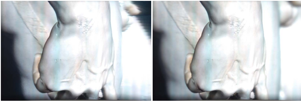
Figure 6: Depth-of-field blur. Left: rendering quality for object portions too far from the screen surface is insufficient because of limited spatial accuracy and precision in calibration. Right: An image-based depth-of-field blur is applied to reduce the effect of depth compression and to adapt scene frequency content to the light field display spatial resolution.
