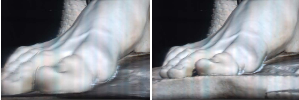
Figure 5: Depth compression. Left: rendering quality for object portions too far from the screen surface is insufficient because of limited spatial accuracy and precision in calibration. Right: non-linear depth compression reduces artifacts while minimizing modification of shape in the neighborhood of the screen surface.
