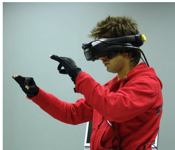
Figure 1 – User wearing left and right hand 5DT- 14 dataglove ultra, plus head, left hand and right hand 6DOF motion trackers. A Cybermind see-through HMD is also worn to visualize the virtual contents onto the surrounding scene.
