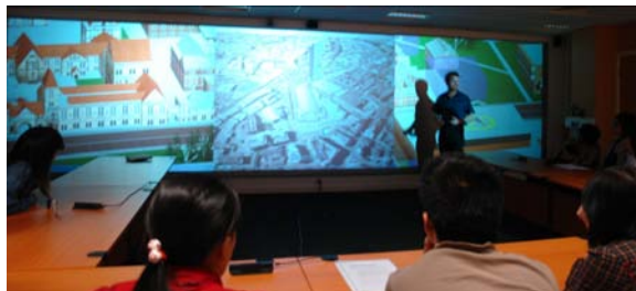
Figure 5: Google Earth projected stereoscopically within the conference node with added layers of three dimensional objects superimposed at the correct position.
