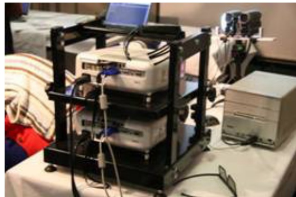
Figure 9: Portable system being exhibited, consisting of two projectors powered by a compact PC shuttle system creating a combined two- and three-dimensional presentation facility.
