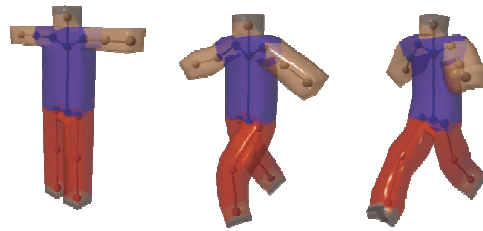
Figure 1: A deformable human model with 4822 elements and a hierarchical skeleton structure of 48 DOFs is computed in real-time with a walking motion animation created by key frames.
