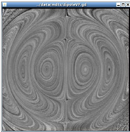
Figure 1: Vector field generated by an irradiating dipole antenna, visualized using our implementation of the fast LIC algorithm and a white noise input layer.
