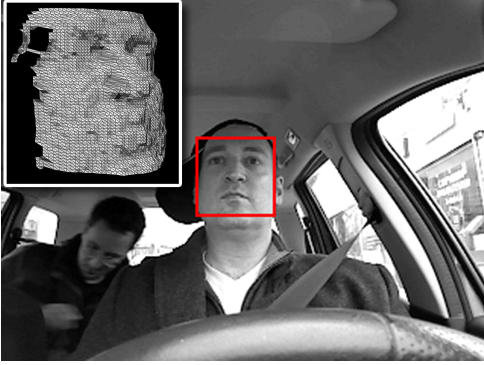
Figure 3: Driver face detected in the color stream (converted to gray). Corresponding 3D data shown top left.
