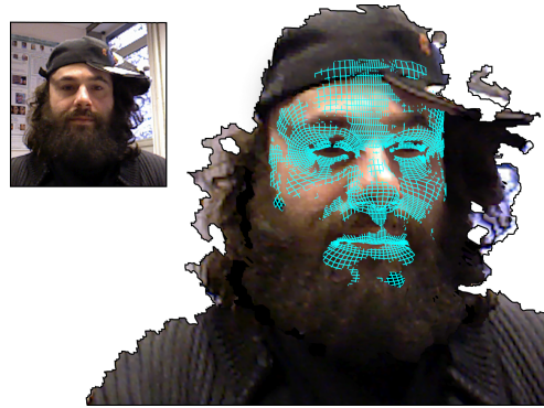
Figure 8: Identity Model successfully tracked to the noisy sensor data despite occlusion due to facial hair.
