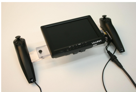
Figure 9: Hydra Controllers with mounted monitor.
