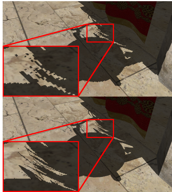
Figure 5: Increased shadow map precision thanks to a smaller light frustum. Without frustum reduction (top) and with a tight camera-dependent frustum (bottom). The differences are most noticeable on thin geometry such as leaves.
