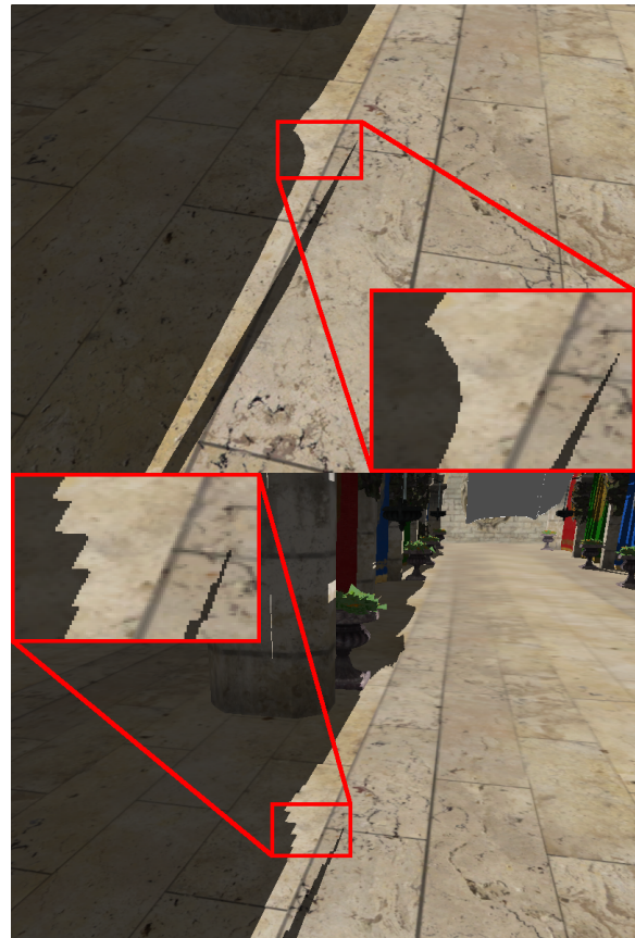
Figure 7: Sudden change of shadow aliasing. Only a small portion of the scene is seen in the first frame (top) and when the camera moves only slightly, the frustum is suddenly much larger (bottom).
