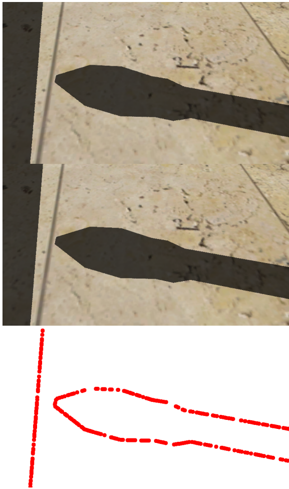
Figure 6: Possible misalignment due to reduced resolution. 4096x4096 shadow map (top), reduced to 1920x1520 shadow map (middle) and marked pixel differences with red dots (bottom).
