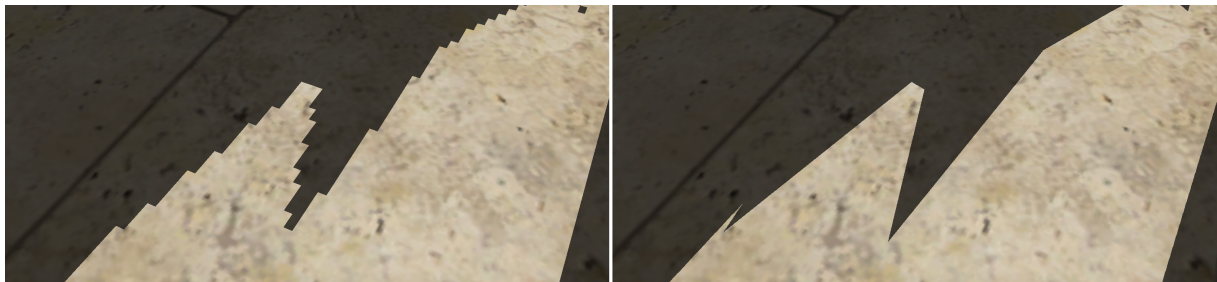
Figure 1: Our new method outperforms standard Shadow Mapping by dynamically reducing shadow map resolution. We improve on quality as well as performance. Standard Shadow Mapping at 4096x4096 (left, 2.8 ms) and our method with resolution reduced to 2700x2300 (right, 2.4 ms).
