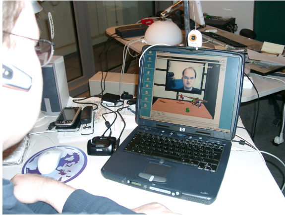
Figure 4: Using the videoconferencing interface the expert can share the view of the designer. He can communicate with the remote participant and guide him using voice communication or instruct the system directly using its speech interface. (Microsoft's NetMeeting / Windows XP)
