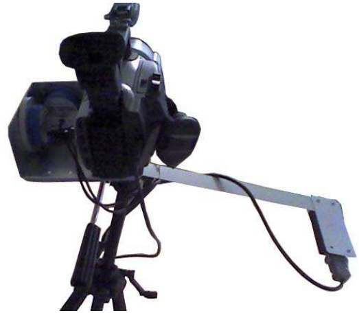
Figure 2: The first approach to the camera tracking, with two inclinometers and a magnetometer, was successful in ground tests and over helicopters, but insufficient for airplanes.
