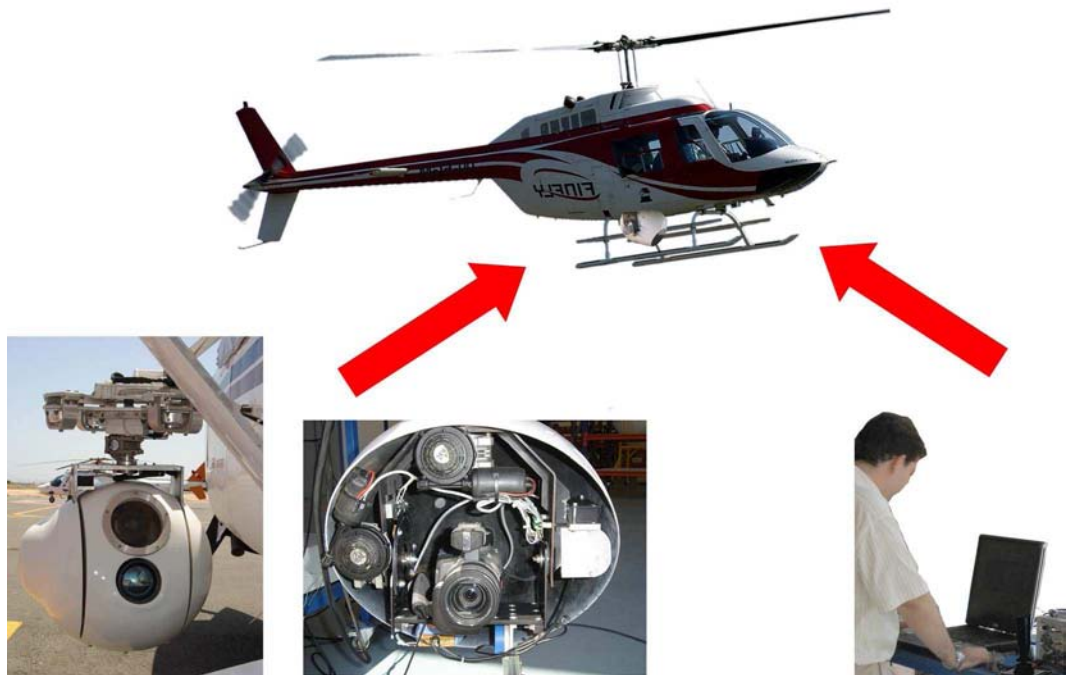
Figure 8: The main hardware components of the AR solution. A GPS and a video camera, controlled by a joystick, are already existent elements and very common on aircraft used for forest fire fighting. A tracking device and a PC with touch-screen are the only new additions to the system.
