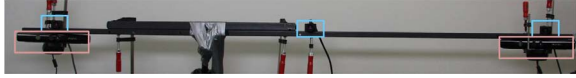
Figure 1: Hardware setup. The two Kinect depth cameras are circled in pink and the three color cameras in blue.
