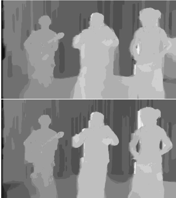
Figure 7: Disparities obtained from the globally optimal geometric image registration step. Top: Result for uncorrected colors. Bottom: Result after registration with the proposed method.
