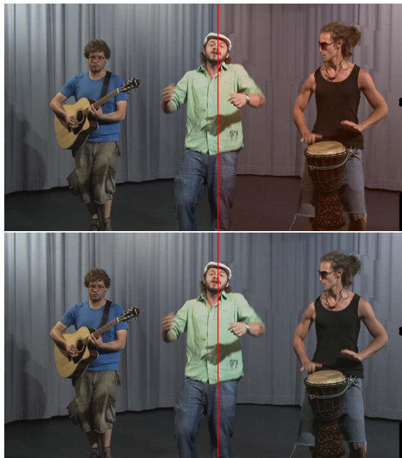
Figure 6: View synthesis based on the scene in figure 5. Both syntheses are composed from the left image of figure 5 on the left of the red line and from the right image on the right of the red line. The synthesis on top is based on the synthetically deviated colors and the synthesis on the bottom is performed after a correction with our registration algorithm.
