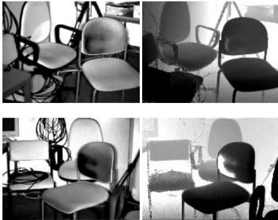
Figure 2: The intensity (left column) and depth images (right column) recorded by two cameras in a wide-baseline setup.
