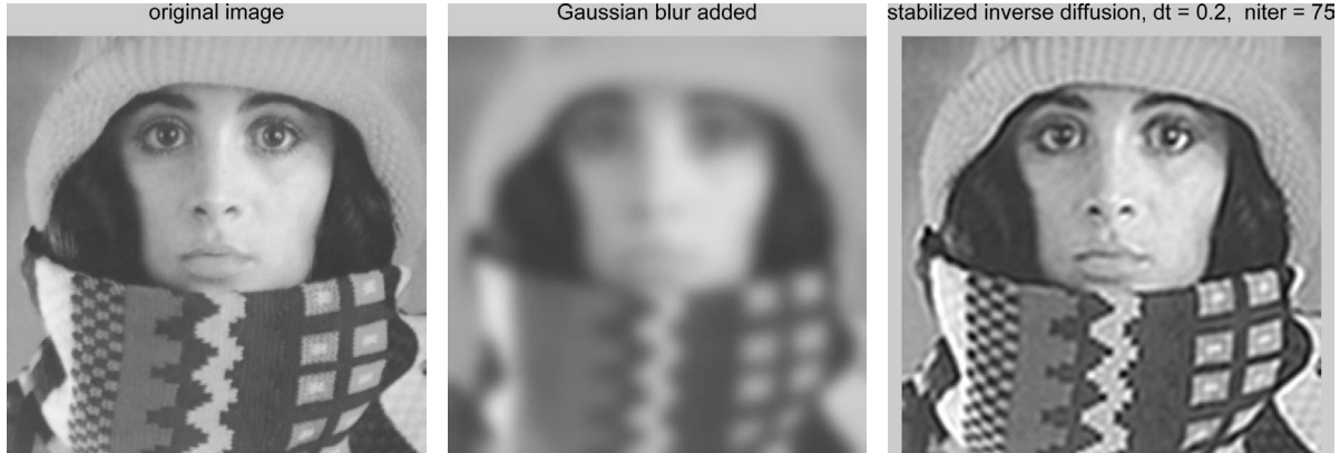
Figure 3: Stabilized inverse diffusion for deblurring Gaussian blur. Left: original image. Middle: discrete Gaussian blur with \sigma = 5 is added. Right: deblurring by (11). See the main text for details.
