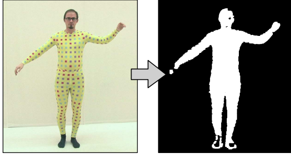
Figure 1: Our segmentation algorithm separates a given image into foreground and background. The foreground area is used as a mask for feature detection.
