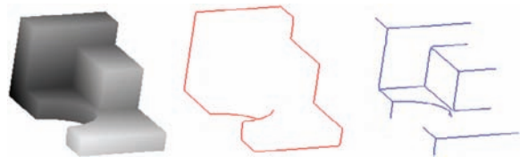
Figure 3: Curve block segmentation using different thresholds to detect step edges (red) and crease edges (blue).
