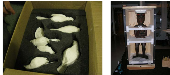
Figure 1: Examples of packaging techniques: (left) cavity packaging and (right) sparse layered packaging. ©Femimore Art Museum and Darla Jackson sculpture blog
