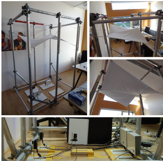
Figure 11: The demo setup for controlled measurement. The sheet is not very stretchable; it is suspended with rubber tapes that can be adjusted manually. The vertical displacement of the scale model corresponds to 2 meters of the real setup (Figures 1 and 2); the sheet deforms significantly. Bottom: The final configuration of the four projectors with the wide-angle camera in the center.
