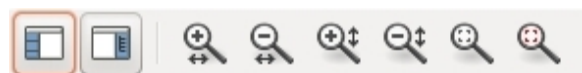
Figure 3: The heatmap view supports several user interactions. From left to right: hide left and right sidebar, horizontal zoom in and zoom out, vertical zoom in and zoom out, zoom to overview, zoom to fit selection.
