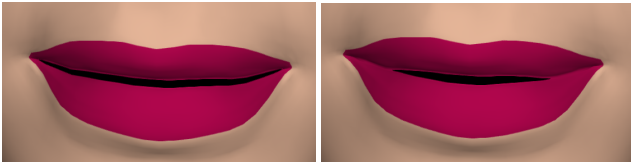
Figure 7: Left: Equilibrium position generated using FEM without stickiness for a small opening of the mouth. Right: The mouth at equilibrium position having been opened the same amount with stickiness: the lips are still connected towards the edges of the mouth recreating the effect shown in the real mouth in Figure 5.
