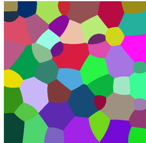
Figure 1: A multiplicative-weighted Voronoi tessellation of 50 sites with random weights between 1 and 5, free of islands and fragmentation artifacts. This 512 \times 512 plot was computed in 2.2 seconds in a 2.5 GHz CORE i5 laptop.
