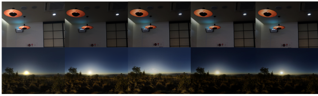
Figure 5: HDR reconstruction results after machine learning from one view of [EKD*17], [SRK20], and [MZCL22] compared with the reference on the left hand side (LDR and HDR images).
